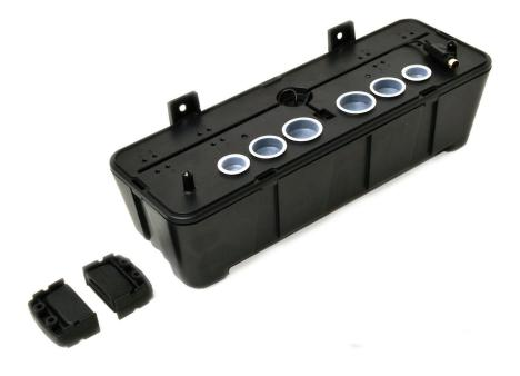
The MultiTank is favoured among architects and design consultants and is available for using with either MegaBlue  $^{\text{\tiny M}}$  or MaxiBlue  $^{\text{\tiny M}}$  pumps. The tank incorporates an energy efficient solid state level sensor which eliminates the use of moving floats - which often become stuck. By manifolding a number of fan coil units into the 1.5L MultiTank, it offers the installer complete flexibility surrounding any multi-unit installation.
