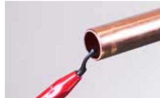
3. Use a pencil type deburrer on internal edges
